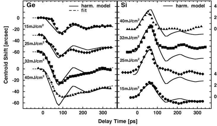
**Fig. 1.** Time dependent shift of the centroid of the measured rocking curves in the Ge-overlayer (left) and in the Si-substrate (right) for different fluences. Solid lines: harmonic model; dashed lines: anharmonic fit.
